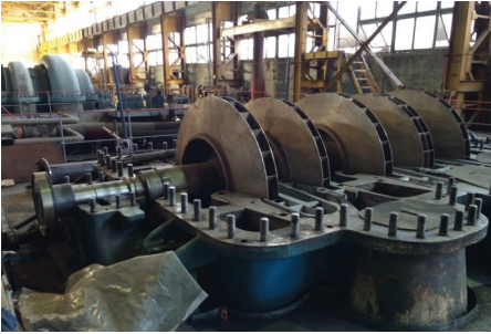
Fig. 1. Damage to the wheels of the 1st – 4th stages of the compressor.
